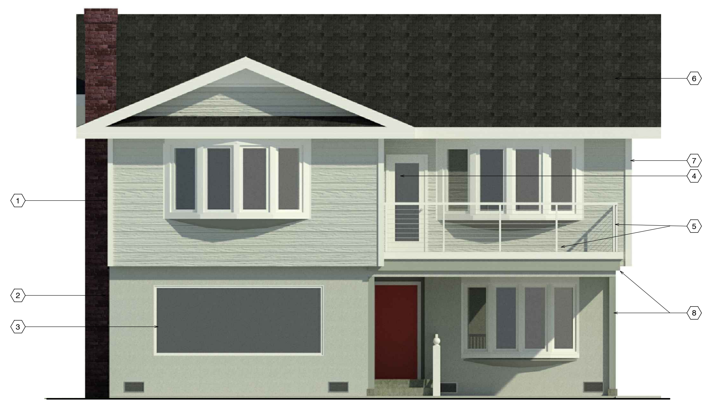
STREET / NORTH ELEVATION (NEW) ADDED LIVING ROOM WINDOW @ 1ST. FLOOR AND ADDED DECK @ 2ND. FLOOR SCALE: 1/4" = 1'-0"
